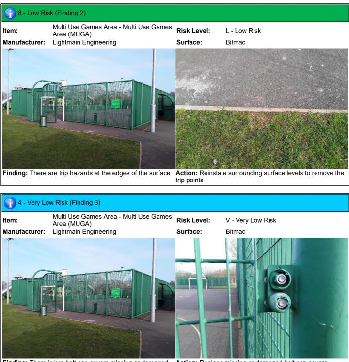
**Finding:** There is/are bolt cap covers missing or damaged on the item
